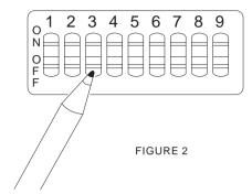
To gain access to the switch, remove the top section of the cabinet, if you have not already done so, Using a pencil, or other similar device, move the code switches to set your house code. Positions one through nine on most MULTI-CODE transmitters are used to set the house code. NOTE: THE MULTI CODE 4120 TWO CHANNEL TRANSMITTER OR 4140 FOUR CHANNEL TRANSMITTER REQUIRES A DIFFERENT CODE SELECTION. REFER TO THE APPROPRIATE INSTRUCTIONS IF THERE IS ANY DOUBT AS TO CORRECT SETTING.
