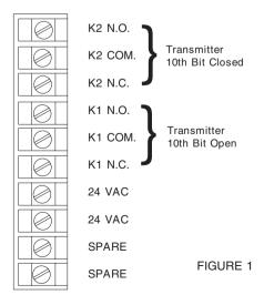
Back the screws on the terminal block off slightly and insert your wiring lugs (or wire) under the appropriate set screw.
