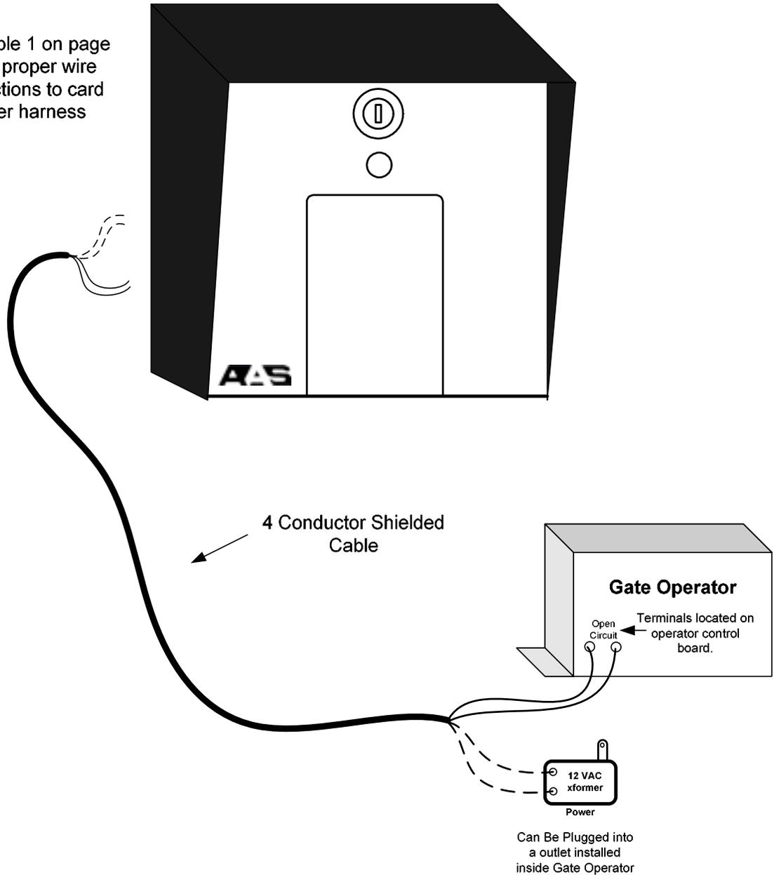
White night light leads will hook directly to power leads when using 12 VAC transformer. If using 24VAC operator control voltage you MUST connect a 100 ohm 10 watt resistor in series with on of the white night light leads to reduce voltage to 12 volts
