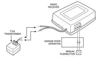
**STEP 4** Test receiver. Be sure the door or gate area is clear. Activate each transmitter and verify that the receiver triggers the operator. If desired, a continuity meter may be used to test the relay contact closure.
