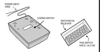
**STEP 2B** Connecting receiver (using operator power). Connect the receiver to the garage door or gate operator as shown in the diagram. Power will be supplied from the operator.
