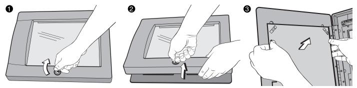
**Mounting Directory:** Pull power supply wiring through center hole on the back of the directory. Mount directory to either a wall or a gooseneck. **NOTE:** If you are mounting to a wall you must punch out the wall mount holes.
