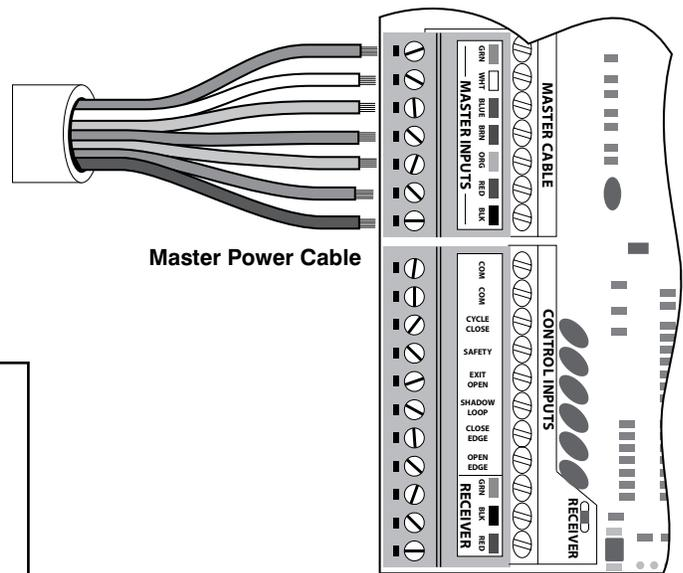
**NEVER** splice wires together. Splicing permits corrosion and seriously degrades the wire's ability to carry an adequate current.
