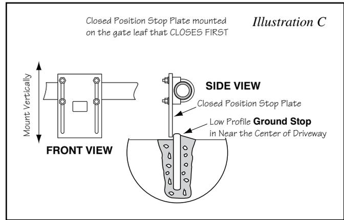
**At this stage of the installation, the operators should be installed on the gate leaves and closed position stops should be in place.**
