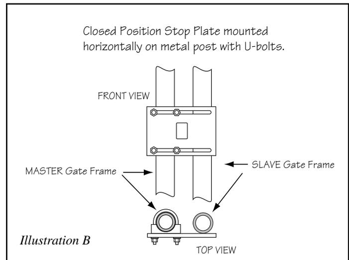
**NOTE:** The optional ground stop post is used to provide a secure point for the SLAVE gate to close against. If you will be using the GTO/PRO Horizontal Gate Lock accessory with your gate operator system, the closed position ground stop is **REQUIRED**, as shown in Steps 2 and 3 on the next page.
