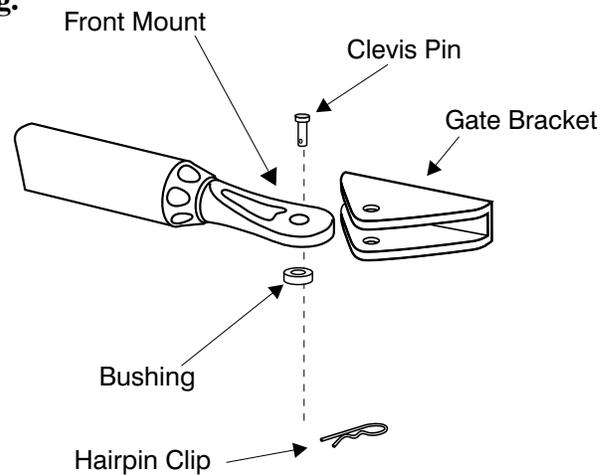
**NOTE:** Substitute a **Pin Lock** for the clevis pin on the front mount of the gate operator to prevent unauthorized removal of the operator from the gate (see *Accessory Catalog*).
