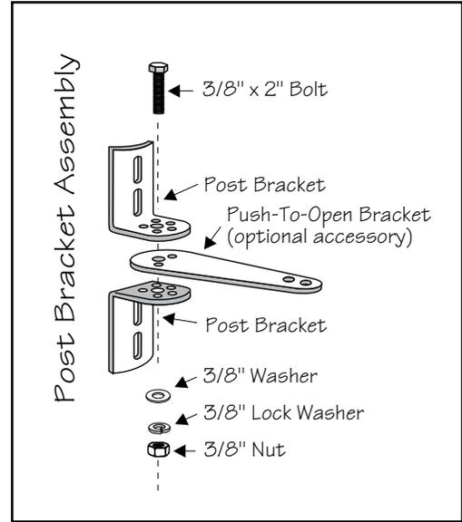
**IMPORTANT:** While determining the mounting point for the post pivot bracket assembly be sure that the position allows for maximum clearance between the gate and the opener in both the open and closed positions, as shown in the diagrams below. This clearance will give the opener the most efficient leverage point for opening and closing the gate and more importantly provides the least possible pinch area.
