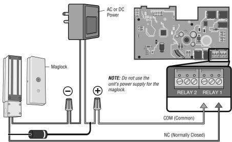
**NOTE:** For DC power install a 1N4001 diode or equivalent.
