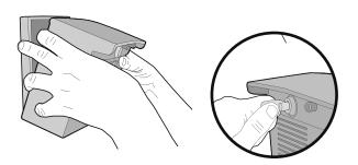
**NOTE:** DO NOT push the top of the unit onto the back panel before the bottom of the unit is in place.
