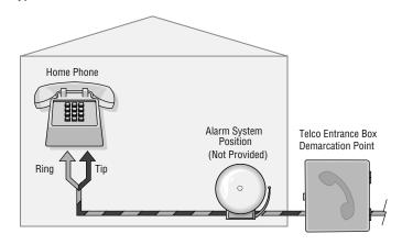
**NOTE:** If the unit will be connected with an alarm system, you must connect the telephone line to the alarm system first in the series from the Telco box. If the units are not connected in this order, they will not operate properly.
