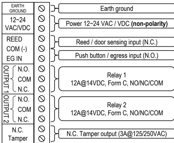
**Earth ground terminal:** Connect a continuous wire from the Earth Ground terminal to a grounding point to avoid damage from static discharge. **If using an AC adapter for power input, do not connect the AC adapter output to Earth Ground.**
