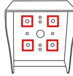
These holes are used to mount the keypad to a gooseneck stand.
