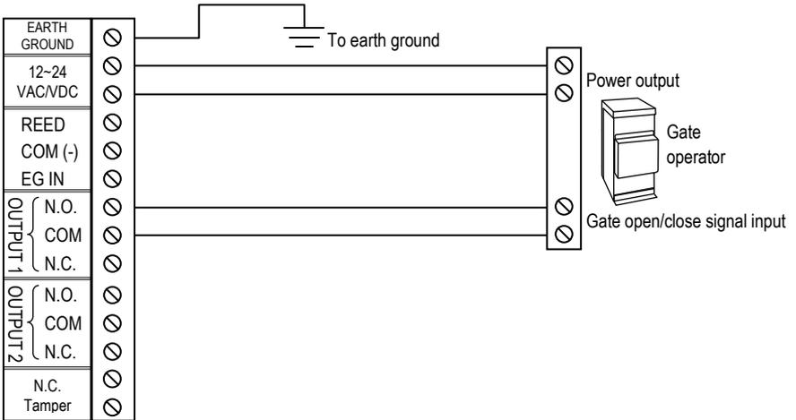
1. Run a continuous wire from the earth terminal to earth ground. For more details, please see page 4, *Earth Ground Terminal*.
