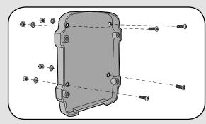
Choose mounting location for Keypad. Remove the back panel and attach it to a solid surface or post.
