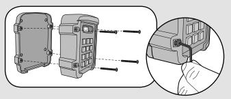
Mount the Keypad onto the back panel with screws. Tighten screws with Allen wrench.
